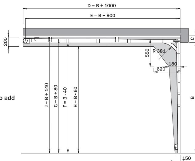
EN A - opening width max. 5 500mm (from door width 4 950mm there is necessary to add the weight of the struts, number of struts equals the number of the sections, strut weight 1,25 kg/m, weight of the section 12kg/m<sup>2</sup>)
